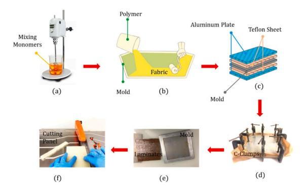
**Scheme** (a) Mixing of monomers (b) lamination of fabrics (c) laminate sandwichched in the mold with aluminum plates covering (d) C-clamping to exert pressure on laminate, (e) demolding the sandwiched laminate after thermal curing, and (f) cuttingof panels into rectangular beams
