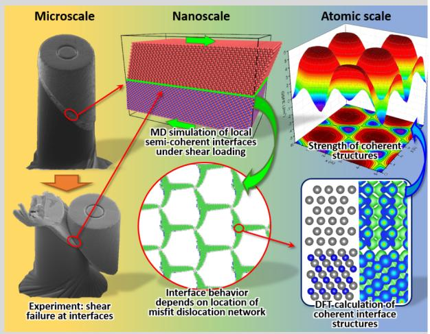
Image: To understand how metal/ceramic interfaces fail under stress, researchers custom-fabricated pillars approximately the thickness of human hair (~100 microns) containing the interfaces studied,
