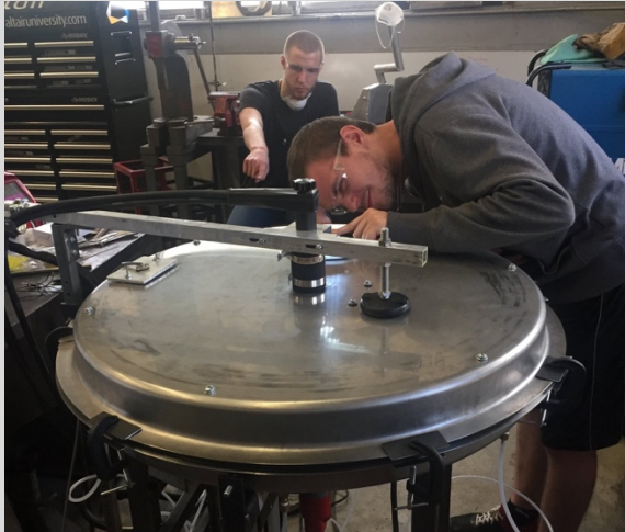
Louisiana State University Mechanical Engineering students designed a rig for making metal 3D printing powders. Aaron Alford (front) inspects the metal powder rig while Michael Guidry offers suggestions. Credit: Dr.Shengmin Guo, Louisiana State University, squo2@lsu.edu
