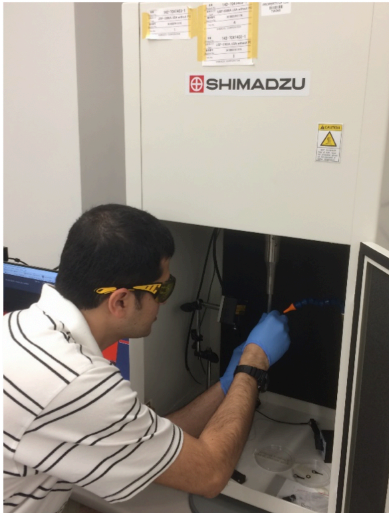
Louisiana State University graduate student Hamed Ghadimi working with SHIMADZU USF-2000 ultrasonic fatigue testing system.
