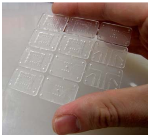
Fig. 13: Molded and fly-cut chips ready for assembly.
