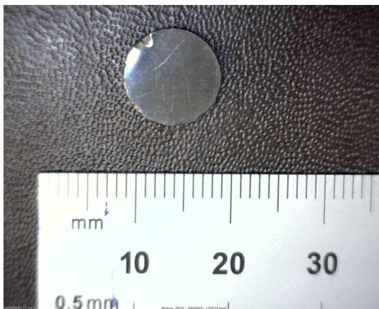
Fig. 4 Pellet of \text{Bi}_2\text{Te}_3 consolidated from ball-milled powder. The powder was pressed in a uniaxial press under a pressure of 50 MPa at 400°C for 1 hour.
