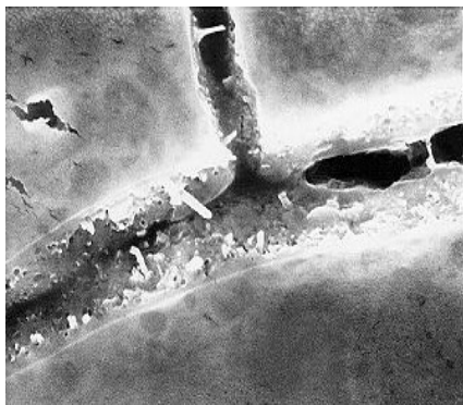
Fig. 1. SEM micrograph of paint scratch containing 5 wt % of halloysite nanotubes in it
