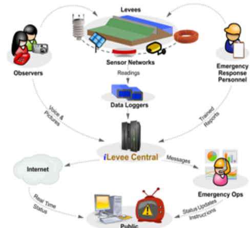
Figure 1. Concept of the iLevee System (Taken from the Proposal)
