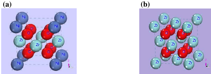
Figure 1. (a). The Ni doped at a substitution site with a Zr vacancy; and (b) pure \text{ZrO}_2 unit cell. The blue sphere stands for Ni atoms, the light green sphere represents the Zr atoms, and the red sphere stands for oxygen atoms.
