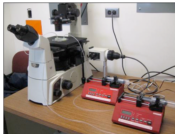
Figure 3. Complete dual pump flow chamber system installed in the laboratory.
