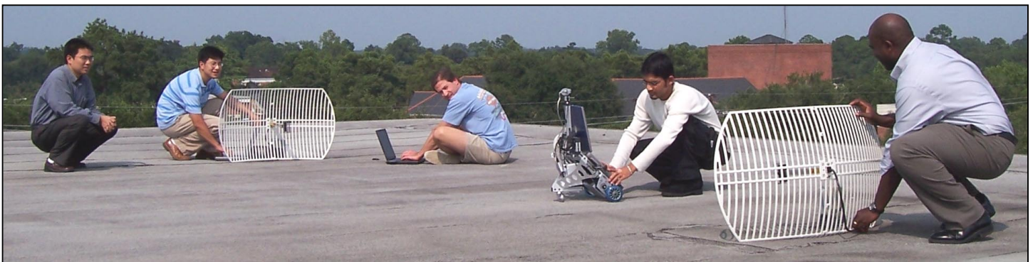
ULL researchers testing wireless communication equipment to be deployed for the powerful ubiquitous computing and monitoring system funded by the DOE EPSCoR program are, left to right, Haining Chen, Dr. Hongyi Wu, Denvil Smith, Atif Siddiqui and Dr. Dmitri Perkins. Chen, Smith and Siddiqui are graduate assistants.
